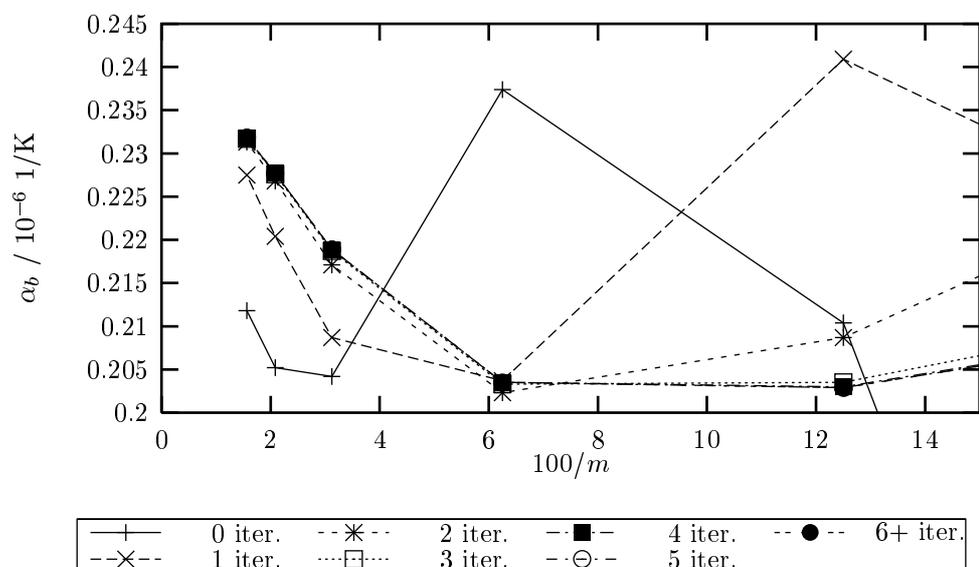
**Figure 4.** Calculated value of  $\alpha_b$  for crystalline orthorhombic polyethylene at 5 K as a function of mesh size. The full line shows results obtained using uniform grids of cell centres. Others use finer meshes in inner regions of the FBZ, with the number of iterations indicated.
