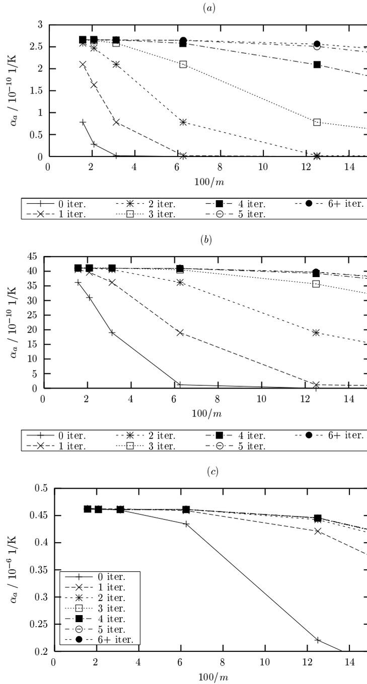
**Figure 2.** Calculated thermal expansion coefficients for the  $a$ -direction ( $\alpha_a$ ) of crystalline orthorhombic polyethylene as a function of mesh size  $1/m$ : (a) at 0.4 K; (b) at 1 K; (c) at 5 K. Full lines are the results from a uniform grid of cell centres as described in the text. Others use finer meshes in inner regions of the FBZ, with the number of iterations indicated. On the right of the figure the lines are directed towards points given by  $m = 4$ .
