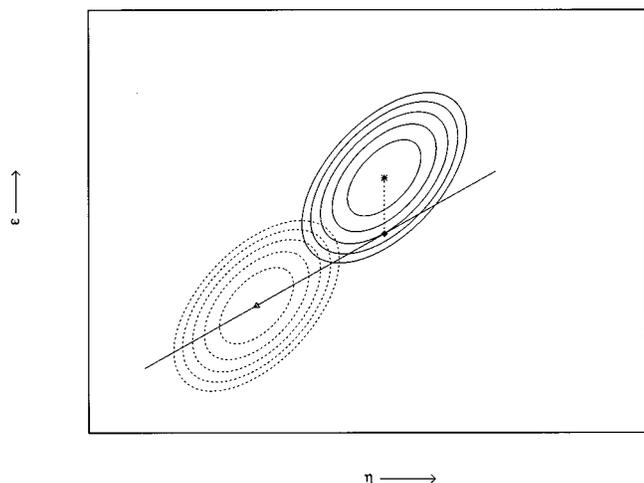
FIG. 1. Energy contours for a system with one external and one internal strain.  $\cdots$ ,  $E^{\text{st}}$ ;  $—$ ,  $F$ . The continuous line shows the states of strain allowed by ZSISA. The point  $\Delta$  marks the equilibrium state of strain of the static lattice, the point  $*$  the true equilibrium at temperature  $T$  and the point  $\blacklozenge$  the state of strain given by ZSISA.
