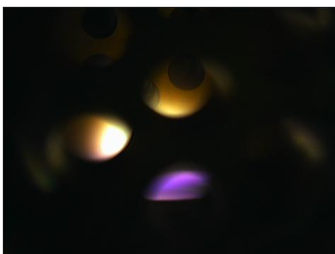
**Figure F.3:** Side image of plasma sustained with a gas composition of 2%  $\text{CH}_4$ ; 7 % Ar; balance of  $\text{H}_2$  at a pressure of 150 Torr sustained at 1.5 kW.
