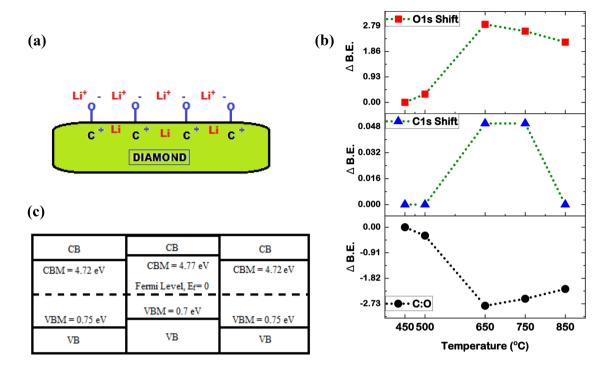
**Fig. 5** a O–C dipole representation of the diamond surface showing the dipole between C–O due to charge transfer between the species. **b** O 1s, C 1s, and C:O relative shifts showing a saturation point at 650 °C and significant changes at 850 °C as explained. **c** The band
