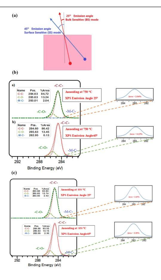
**∢Fig. 3** a Angle-resolved XPS showing Bulk sensitive (BS) and surface sensitive (SS) modes at 25° and 45° to the normal of the sample. **b** Angle-resolved XPS of C1s peak in the BS mode (25°) and SS mode (45°) at 750 °C. **c** Angle-resolved XPS of C 1s peak in the BS mode (25°) and SS mode (45°) at 850 °C
