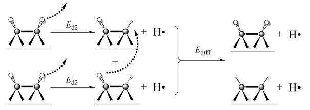
**Figure 4.** Proposed desorption path for hydrogen on the <100> surface of single-crystal diamond. Hydrogen desorbs from the fully terminated dimer with a desorption energy of  $E_{d2}$  = 3.51 eV, generating a partially terminated dimer and a hydrogen radical. Then, another hydrogen from a partially terminated dimer diffuses ( $E_{diff}$ ) across the surface to form a fully terminated and an unterminated dimer. Dark circles represent carbon atoms, while white circles represent hydrogen atoms.
