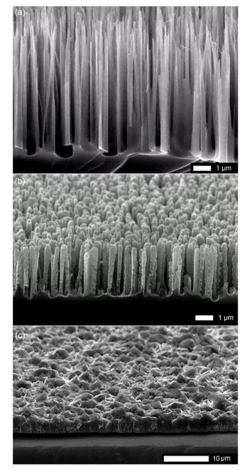
**Figure 1.** SEM micrographs of a) a cross section through a bSi wafer, b) a representative sample of a bD wafer, and c) a 'flat' diamond control wafer (i.e., a uniform, pinhole-free microcrystalline diamond film on a Si substrate).
