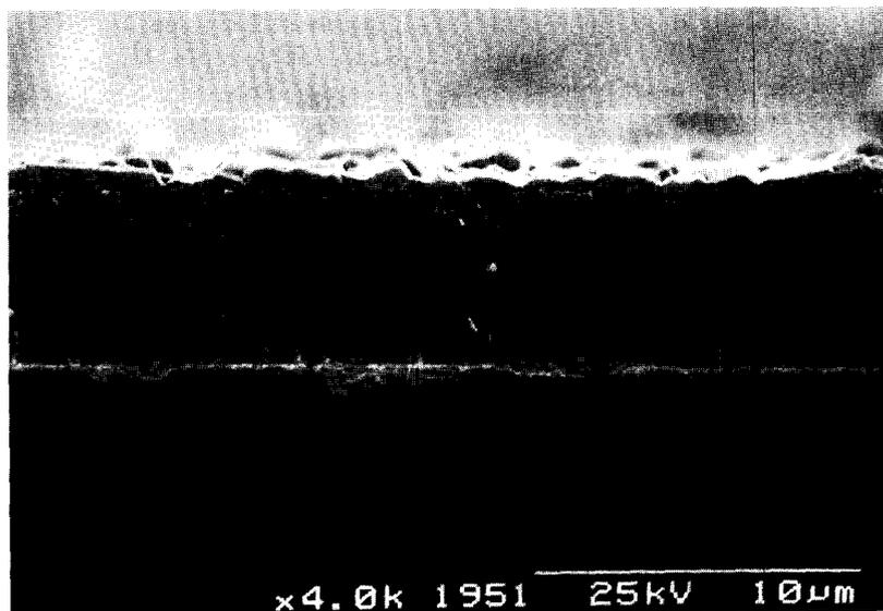
Fig. 2. SEM cross-section of the film in fig. 1 showing columnar growth structure.
