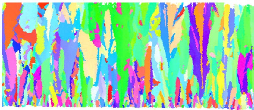
Fig. 3. 3D tomographic electron backscattered detection images of the cross-section through a CVD diamond film grown with 1%CH 4 /H 2 at 900 °C (from the Max-Planck-Institut für Eisenforschung). The orientations of different grains have been colour-coded based upon their alignment with the axis parallel to the growth direction. Reprinted with permission of the authors from Ref. [28], copyright 2009, Wiley.
