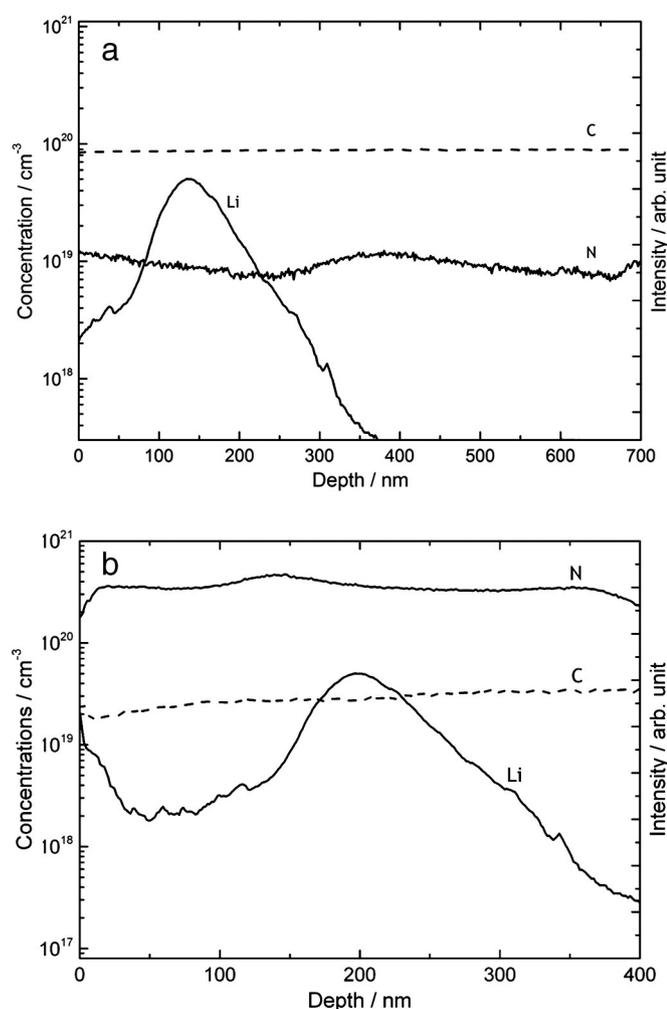
**Fig. 5.** SIMS depth profiles (top 400 nm only) of samples grown with (a)  $\text{N}_2$  gas and (b)  $\text{NH}_3$  gas added to the CVD gas mixture.  $\text{Li}_3\text{N}$  was added after the film thickness was  $\sim 2 \mu\text{m}$ , and then a 200 nm capping layer was added using the same gas mixture as for the lower layer. The concentrations of Li and N are shown on the left-hand axis, while the C intensity is shown on the right-hand axis.
