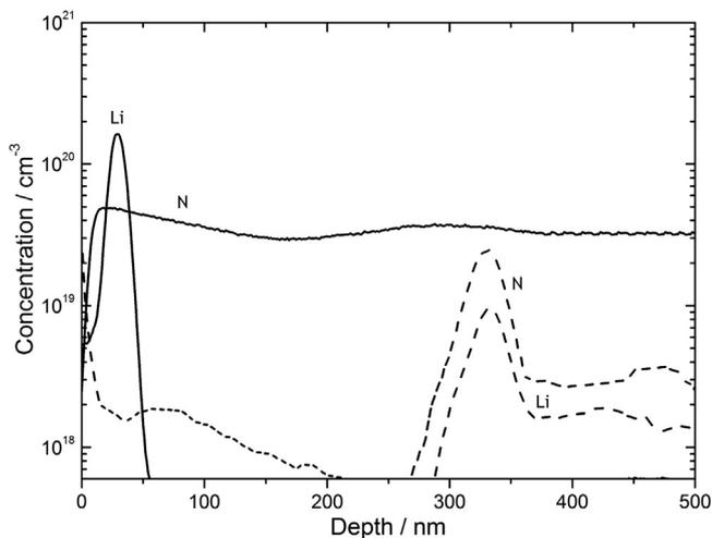
Fig. 7. SIMS depth profiles (top 500 nm only) of two Li–N co-doped diamond films grown on HPHT type Ib substrates using  $NH_3$  (solid lines) or  $N_2$  (dashed lines) as the nitrogen precursors.
