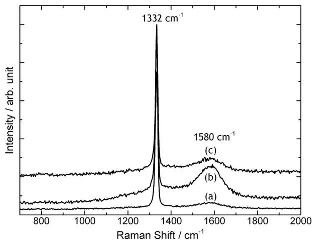
Fig. 1. Laser Raman spectrum (325 nm He–Cd excitation) obtained from different layers of the microcrystalline diamond films grown on Si. (a) Undoped diamond, (b) nitrogen-doped diamond, and (c) Li/N-co-doped diamond.
