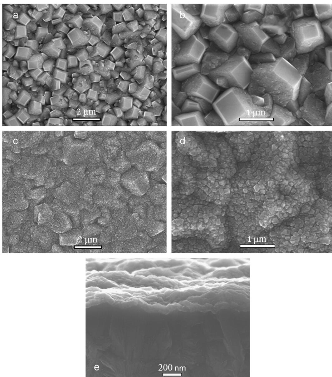
Fig. 2. SEM micrographs showing the morphologies of the two types of diamond films grown on Si substrates. (a) & (b) Nitrogen-doped microcrystalline diamond. (c), (d) & (e) Li–N-co-doped diamond with (e) showing a cross-section through the film.
