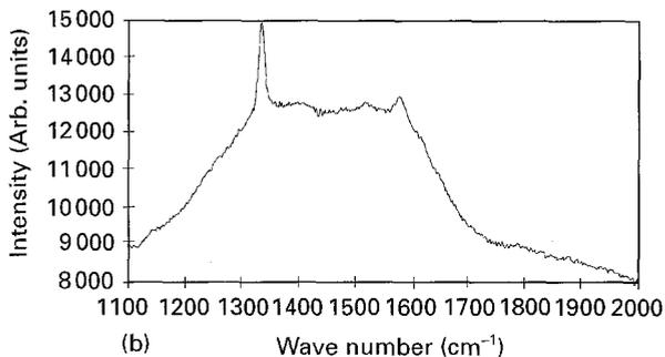
Figure 2 Raman spectra of diamond fibre showing (a) before laser treatment the sharp peak at  $1332\text{ cm}^{-1}$  due to diamond, (b) after laser ablation the additional broad peak around  $1600\text{ cm}^{-1}$  attributed to graphitic carbon.
