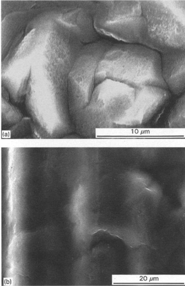
Figure 7 The smoothing effect of laser irradiation on surface diamond facets: (a) initial smoothing, and (b) almost complete smoothing.
