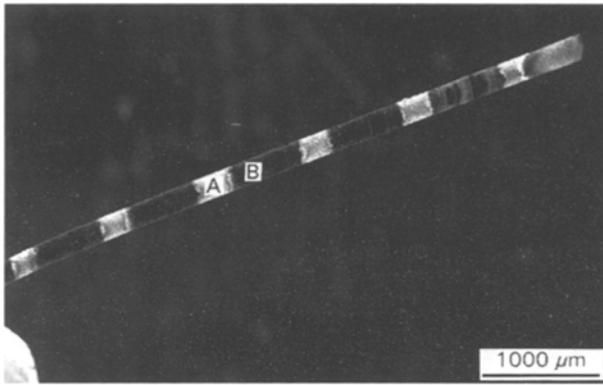
Figure 1 SEM low-magnification secondary electron image of diamond fibre showing a laser irradiated area at B and an unirradiated area at A.
