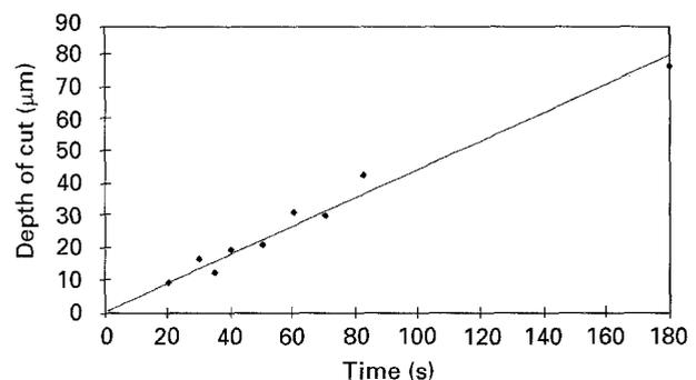
Figure 6 Plot of depth of laser cuts against time for an estimated laser fluence of  $10 \text{ J cm}^{-2}$ .
