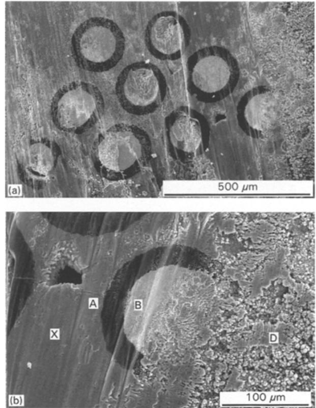
Figure 9 (a) Laser-cut section of composite shown in Fig. 8a, titanium deposited at D from the ablation front, (b) smooth areas extending across titanium-diamond-tungsten phases. Titanium deposited at D from the ablation front.
