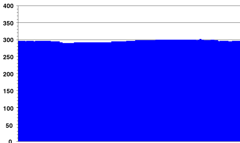
Figure 11. Simulated cross-section of a diamond film grown using the standard conditions given in table 1 but with \beta -scission turned off ( P_{\text{beta}} = 0 ), for a 600 \times 400 grid and blocks of size 2 \times 2 .
