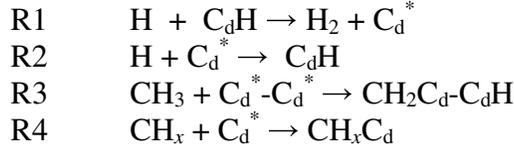
Depending upon which C<sub>1</sub> species adds to the substrate, there are different rate laws (with correspondingly different rate constants<sup>10</sup>) which govern the kinetics, and hence the growth rate. It is possible to estimate the contribution to the growth rate, *G* (in μm h<sup>-1</sup>), of the important C<sub>1</sub> species, using formulae stated in Ref. 17:
