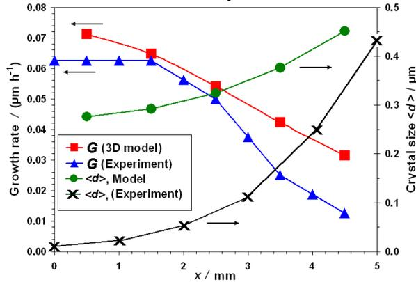
**Figure 3.** Total growth rate and average crystal size calculated as a function of distance  $x$  from the center of the substrate.
