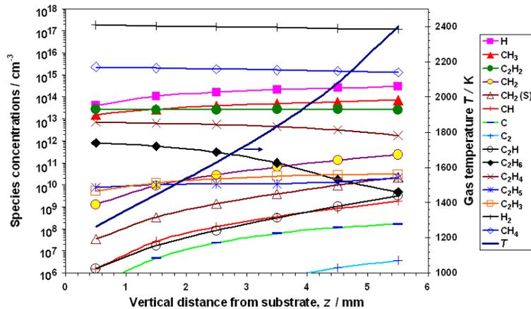
**Figure 2.** Concentrations of various gas phase species as a function of  $z$ , the vertical distance between the substrate centre ( $z = 0$ ) and the filament ( $z = 5.5 \text{ mm}$ ), as well as the variation of the gas temperature,  $T$ . The calculation was performed using values of  $Q$  and  $\Delta T$  so as to fit the experimental growth rates.
