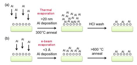
**Figure 1.** a) The thick-film method deposits a thick metal layer onto O-terminated diamond, and excess metal is washed off, leaving a (sub)monolayer of metal chemically attached to the surface. b) The thin-film method deposits a (sub)monolayer of metal that is "activated" by thermal annealing.
