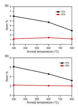
**Figure 8.** Atomic percentages of surface O and Al for Al + O-terminated a) (100) and b) (111) diamond prepared by electron beam evaporation. For both O and Al, a surface coverage of  $\approx 6$  at% corresponds to one ML.
