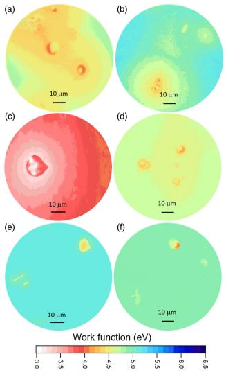
**Figure 10.** Color-coded work function maps of Al + O-terminated diamond prepared by electron beam evaporation, at annealing temperatures of a,b) 300 °C, c,d) 600 °C, and e,f) 800 °C. (a), (c), and (e) are for the (100) surface and (b), (d), and (f) are for the (111) surface.
