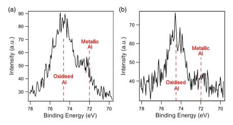
Figure 2. XPS spectra of the Al 2*p* peak for the two polycrystalline Al + O-terminated BDD samples. a) Unannealed sample and b) annealed sample, both prepared by the thick-film process.
