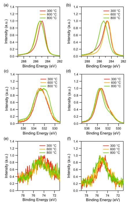
**Figure 3.** XPS spectra of a,b) C 1s, c,d) O 1s, and e,f) Al 2p peaks at different annealing temperatures for thick-film-prepared Al + O-terminated diamond. (a), (c), (e) are from the (100) surface, and (b), (d), (f) are from the (111) surface. The peak heights have all been normalized to the same maximum intensity.
