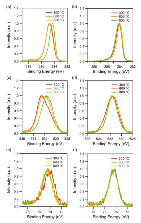
**Figure 9.** XPS spectra of a,b) C 1s, c,d) O 1s, and e,f) Al 2p peaks at different annealing temperatures for Al + O-terminated diamond prepared by electron beam evaporation. (a), (c), and (e) are from the (100) surface, whereas (b), (d), and (f) are from the (111) surface.
