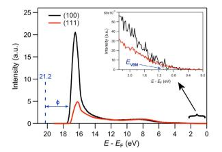
**Figure 5.** UPS spectra (He I excitation at 21.2 eV photon energy) acquired after a 300 °C anneal for AI + O-terminated (100) and (111) single-crystal diamond prepared by the thick-film procedure. The analyzed region is  $\approx 200 \, \mu m^2$ . Inset shows a magnified view of the fitting used to determine the VBM energy relative to the Fermi energy.
