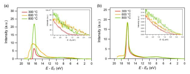
Figure 11. UPS spectra (He I, 21.1 eV photon energy) of AI + O-terminated a) (100) and b) (111) diamond prepared by electron beam evaporation. Inset shows a magnified view of the VBM energy relative to the Fermi energy.
