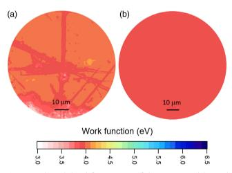
Figure 6. Color-coded work-function maps of Al + O-terminated diamond prepared by the ALD procedure after annealing at 300  $^{\circ}$ C for a) the (100) surface and b) the (111) surface.
