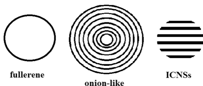
Fig. 1. Schematic representation of carbon nanospheres.
