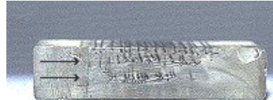
Figure 5. A cross-section through one of the PMCs, showing two layers (indicated by the arrows) of 15 diamond fibres each equidistant from the centre of the block.
