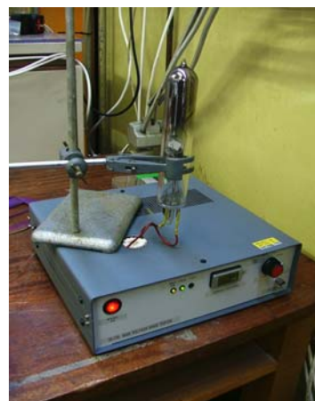
Fig. 4 Bottle testing using a pulsed DC diode test kit
