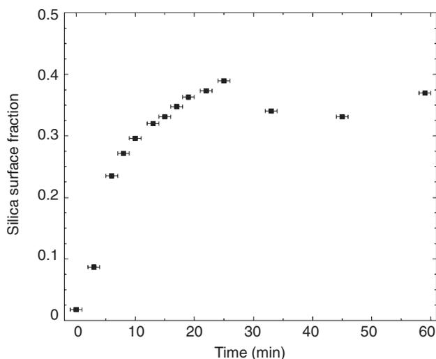
FIG. 8 Silica surface fraction as a function of drying time, which is taken from the first appearance of silica in the ESEM images.
