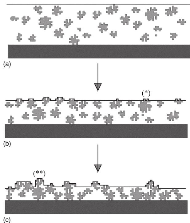
FIG. 6 Schematic of silica in aqueous lacquer during drying. Stage I of latex film formation corresponds to (a), where the silica is dispersed throughout the aqueous latex suspension; (b) and (c) are the results of stage II and III (or II\*) of latex film formation, respectively.
