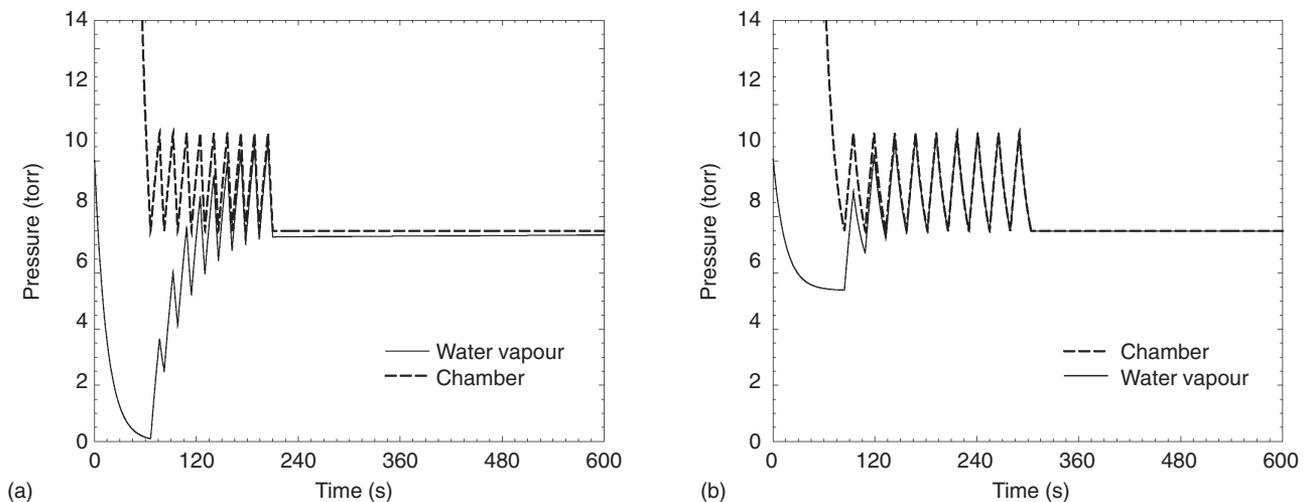
FIG. 3 Water vapour and air pressure as a function of time during the optimised pumpdown of Cameron and Donald (1994) (a), and with a water source within the specimen chamber (b).
