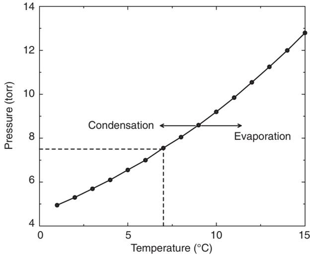
FIG. 2 The saturated vapour pressure line for water, in the ESEM pressure range. The condensing and evaporating regimes are shown. Dotted lines show the conditions used in this experiment, 7.0°C and 7.5 torr (1 atm=760 torr).
