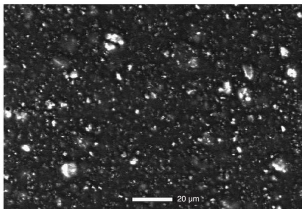
FIG. 7 Environmental scanning electron microscope image of film dried at room temperature. Exactly the same structure is shown as that for a specimen dried in situ.
