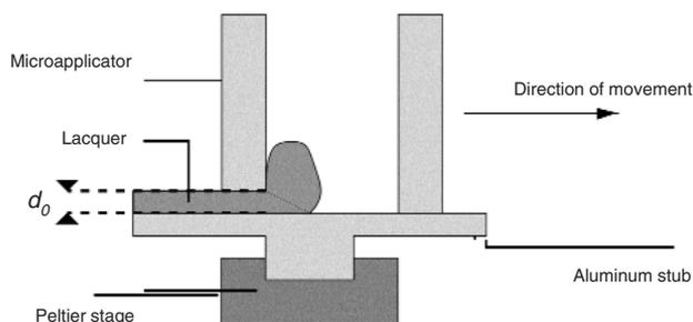
FIG. 4 Schematic experimental set-up. Movement of the microapplicator leaves a wet film of thickness  $d_0$  (200  $\mu\text{m}$ ) on the substrate. The aluminum stub fits snugly in the ESEM Peltier stage.
