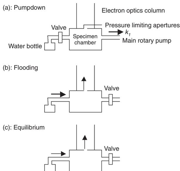
FIG. 1 The three modes of operation of the ESEM vacuum system. Pumpdown (a) is the removal of air and water vapour from the specimen chamber by the main rotary pump; flooding (b) is the injection of water vapour into the specimen chamber from the water bottle; and equilibration (c) is the residual flow of air and water vapour into the electron optics column, matched by an equal flow from the water bottle (Cameron and Donald 1994).
