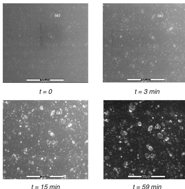
FIG. 5 Lacquer containing precipitated silica undergoing drying in the ESEM. From an aqueous dispersion, the lacquer dries to reveal silica particles. The area (a) shows how an individual particle is revealed over time. Bars=50  $\mu\text{m}$ .
