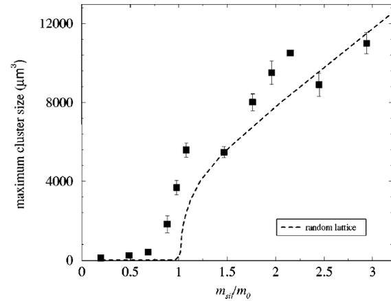
FIG. 10. Maximum cluster size as a function of  $m_{sil}/m_0$ . At the percolation threshold, the maximum cluster size increases discontinuously. Further increase in cluster size is the result of densification. Dotted line is the maximum cluster size on a  $256 \times 256 \times 64$  lattice.
