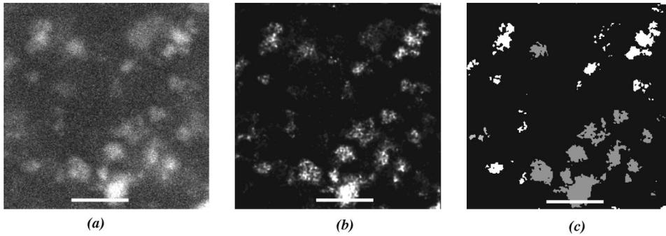
FIG. 2.  $xy$  images of dried lacquer with silica. (a) Unreconstructed image, (b) EM reconstruction with 100 iterations, (c) segmented image with 3D percolating silica structure shown in white, other silica particles in grey. Bars =  $4 \mu\text{m}$ .
