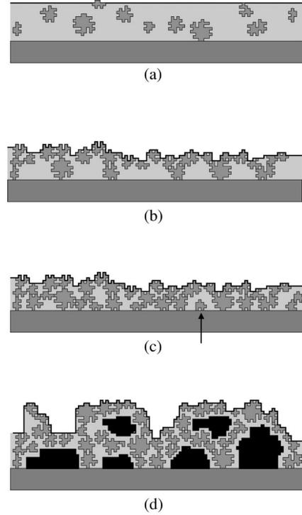
FIG. 1. Schematic of the model of silica structure within dried lacquer. The low concentration regime (a) ( $m_{sil}/m_0 < 1$ ), critical mass of silica (b) ( $m_{sil}/m_0 = 1$ ), and two possibilities for  $m_{sil}/m_0 > 1$ , with silica densification from collapse (c), or void formation with more robust silica (d). Note that (c) does not exclude the possibility of isolated silica particles: for example, that marked in (c).
