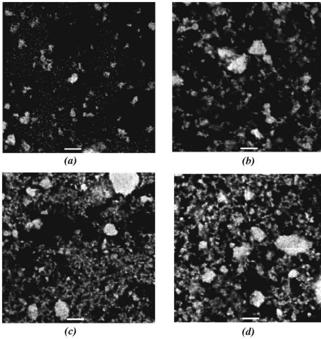
FIG. 6. EM-restored confocal images of film with silica at a range of concentrations. (a)  $m_{sil}/m_0=0.47$ , (b)  $m_{sil}/m_0=0.94$ , (c)  $m_{sil}/m_0=1.87$ , and (d)  $m_{sil}/m_0=2.81$ . All images are  $512 \times 512$  pixel  $xy$  slices taken at a depth of  $7 \mu\text{m}$  from the surface of the film. Faint horizontal and vertical lines in each image are artifacts of EM restoration of each image in four sections, which are then recombined. Bars =  $4 \mu\text{m}$ .
