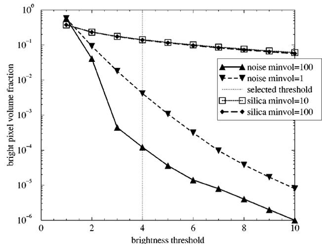
FIG. 3. The selected threshold is the black dotted line, at a brightness of 4. The fraction of bright pixels is shown as a function of threshold. Lines are plotted for images of a silica-containing specimen, and for a specimen without any silica (noise). The minimum cluster volume to be treated as a silica particle is set to 1 and 100 pixels in each case.
