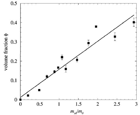
FIG. 7. Silica volume fraction as a function of  $m_{sil}/m_0$ , determined from confocal images. This plot is a direct realization of Eq. (3.10). The value of the packing fraction  $p$  is found with a regression fit.
