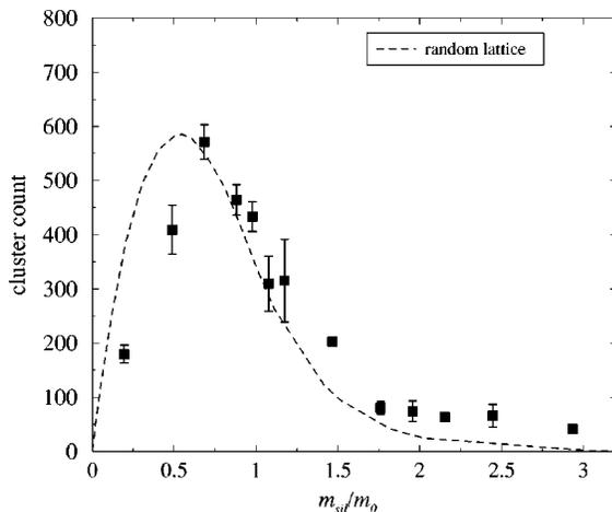
FIG. 9. Cluster count as a function of  $m_{sil}/m_0$ . Dotted line is the count on a randomly populated  $256 \times 256 \times 64$  cubic lattice, normalized to the experimental peak and scaled to  $m_{sil}/m_0$ .
