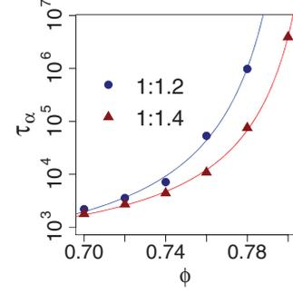
FIG. 5. (Color online) The relaxation time  $\tau_\alpha$  against area fraction  $\phi$  for the two values of  $R$  in the hard disk system.  $\tau_\alpha$  is measured as the time taken by the self-intermediate scattering function to fall to  $\exp(-1)$  [45]. The lines are VFT fits:  $\tau_\alpha \propto \exp[A/(\phi_0 - \phi)]$ .  $\phi_0$  equals 0.82 (0.83) for the  $R = 1.2$  (1.4) systems.
