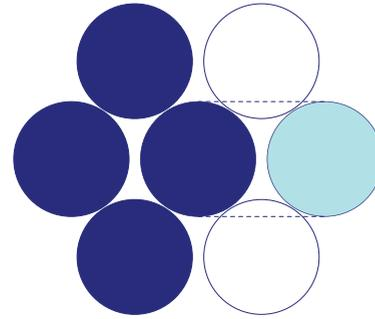
FIG. 1. (Color online) The kinetic constraints in the 2-TLG model: for the central particle to move into the rightmost vacancy it passes through the mutually neighboring sites. These must be empty for the move to be accepted.
