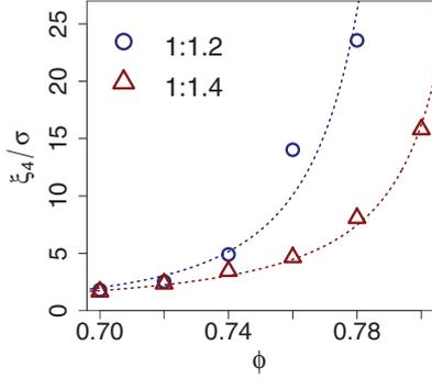
FIG. 7. (Color online) The dynamic correlation length  $\xi_4$  increases with area fraction for both  $R = 1.2$  and  $R = 1.4$ . As with the increase in relaxation time, the effect is greater for  $R = 1.2$ . Lines are a guide to the eye.
