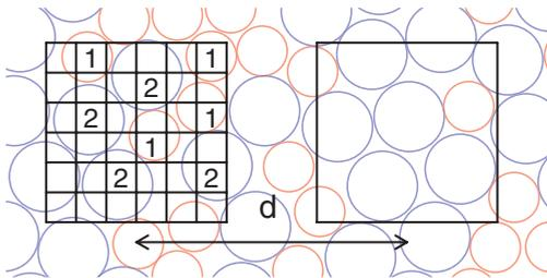
FIG. 3. (Color online) The system for discretizing the patch configuration in the MC hard disk system (not to scale). A grid is superimposed on the patch, and pixels that include a particle center are marked 1 or 2 depending on particle type. Empty space is encoded with zero. The patches are represented by a 3-ary number. Mutual information is measured between two patches separated by a distance  $d\sigma$ .
