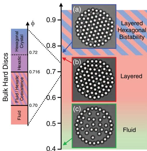
FIG. 2. Colloidal corral phase diagram and illustrative micrographs. At low density the interior is fluid-like (c). On increasing density a concentric layered structure develops (b). For  $\phi_{\text{eff}} \gtrsim 0.77$  there exists a bistability between concentric layered and locally hexagonal configurations (a). Left hand side shows phase behaviour for bulk hard discs at comparable area fractions.<sup>28</sup>
