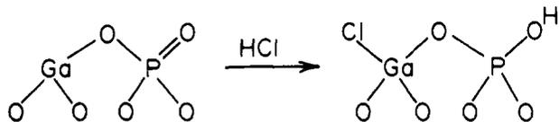
regenerating some terminal P(OH) groups and changing the three-coordinate gallium center to a four-coordinate one, Figure 21. Some hydrogen-bonding of HCl either to the P(OH) groups or to the oxygen part of the framework might be responsible for the band around 3450  $\text{cm}^{-1}$ , by reference to work on proton loaded zeolite Y and  $\text{AlPO}_4\text{-5}$ .<sup>12</sup> It seems that at room temperature the Ga(OH) functionality is behaving as an essentially neutral hydroxyl group.
