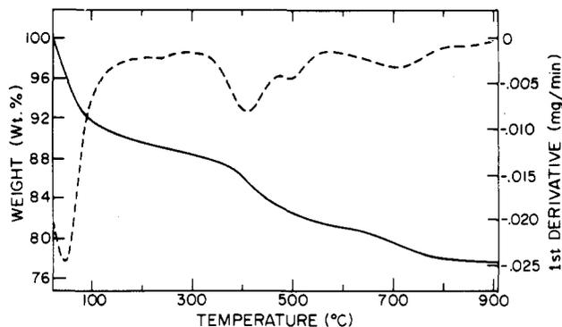
**Figure 4.** TGA/DTG trace of cloverite, run at 1 °C/min, under  $N_2$ .
