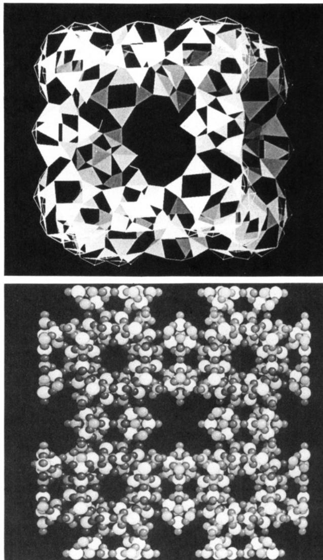
Figure 2. CHEM-X illustrations of cloverite based on the single-crystal atomic coordinates of framework Ga,P,O,F:<sup>1</sup> (A) (top) [100] projection of unit cell and (B) (bottom) the 29–30 Å supercavity.
