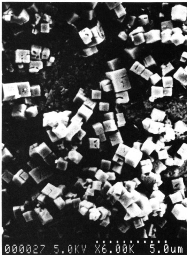
Figure 1. SEM data for as-synthesized cubic cloverite.
