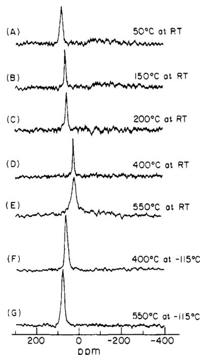
**Figure 13.**  $^{129}\text{Xe}$  NMR of cloverite equilibrated with 400 Torr xenon and pretreated at (A) 50  $^{\circ}\text{C}$ , (B) 150  $^{\circ}\text{C}$ , (C) 200  $^{\circ}\text{C}$ , (D) 400  $^{\circ}\text{C}$ , and (E) 550  $^{\circ}\text{C}$ . Spectra recorded at room temperature and after cooling to  $-115$   $^{\circ}\text{C}$  for samples pretreated at (F) 400  $^{\circ}\text{C}$  and (G) 550  $^{\circ}\text{C}$ .
