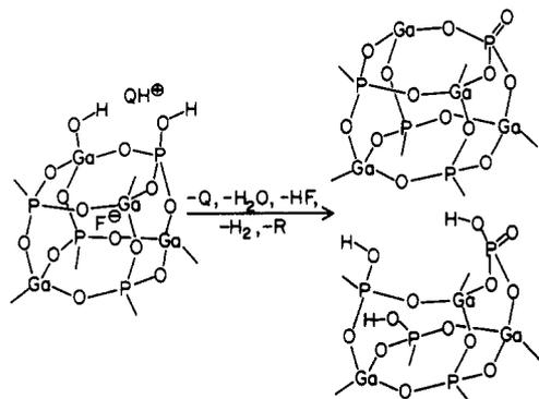
**Figure 21.** Double four-ring thermal chemistry of cloverite proposed to be responsible for the collapse of the interrupted framework: (top right) dehydroxylation–dehydrofluorination and (bottom right) partial fragmentation pathway.
