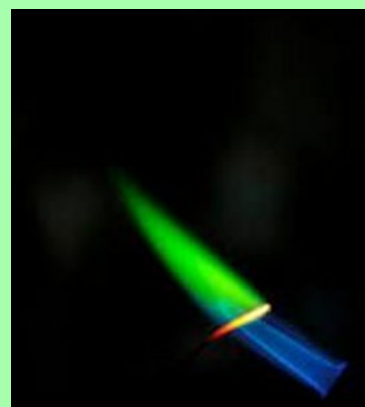
The green flame test for thallium.
