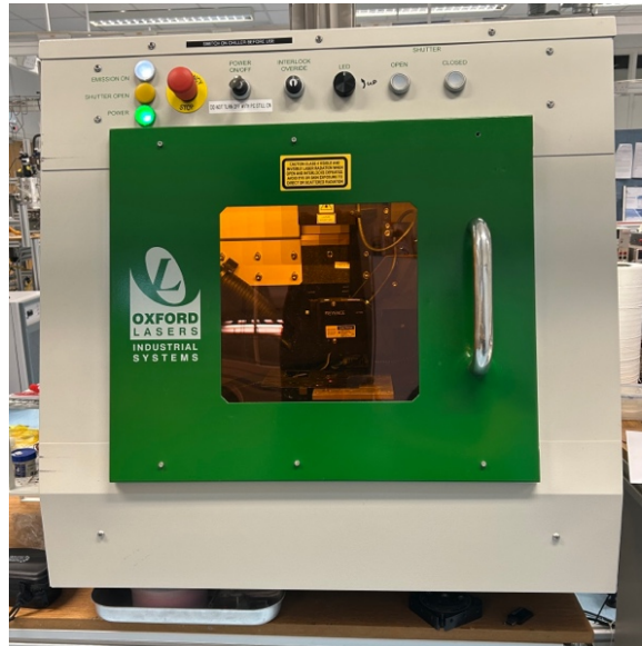
Figure 13: The Oxford Lasers micromachining system used for the membrane process.
