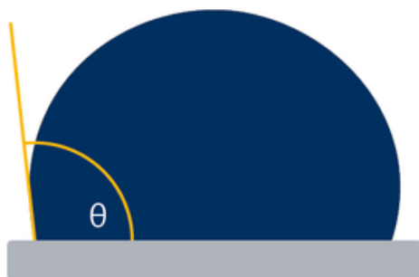
Figure 9: Sessile drop method for static contact angle measurement demonstrating the position of the contact angle when a liquid droplet (blue semicircle) is placed on a solid surface (grey rectangle) 21 .
