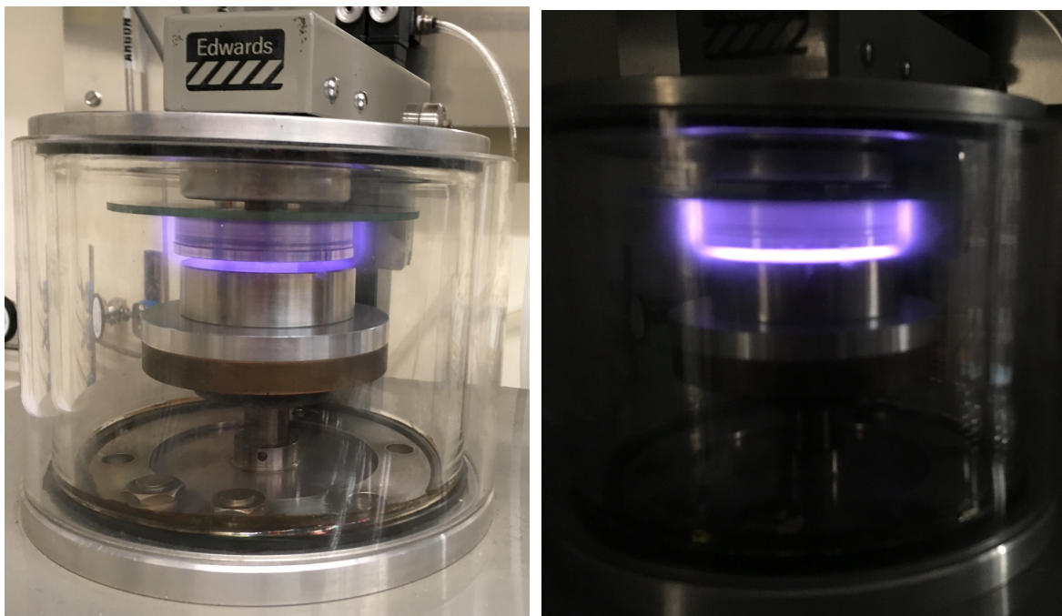
Figure 24: Photographs of the O_2 plasma reactor during operation and hence displaying the self-sustaining glow discharge in the light (left) and in darkness (right).
