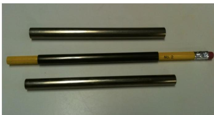
**Figure 12.** Small sections of fuel rod cladding that demonstrate the diameter of the tubing. In an assay in a reactor, these tubes would be 4 meters long. [96]
