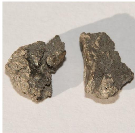
**Figure 6.** Left; some samples of recently cut zirconium [30]. Right; zirconium that has been left open to the air for a year and as a result has developed a thick oxide layer and appears much duller [31].
