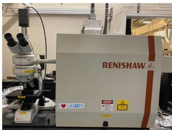
Figure 20 a) A diagram depicting the pathway of the laser and scattered light inside a Raman spectrometer. Created with reference to Ref. 87. b) The Renishaw 1000 Laser Raman Spectrometer in the Bristol Diamond Lab.
