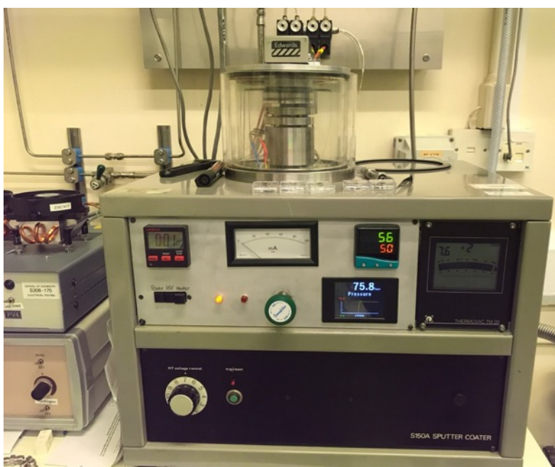
Figure 16: Converted Edwards sputter coater, nicknamed 'The Terminator', used for oxygen termination.
