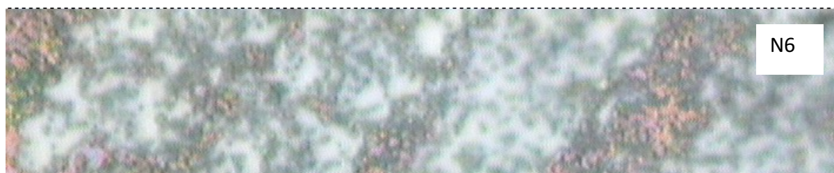
Figure 23: Optical microscope image of N6 diamond film which delaminated from the Mo substrate, shown by the rainbow effect.
