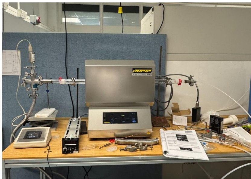
Figure 19 Tube furnace used for N-terminations. On its left is the digital barometer, on its right is the nitrogen input
