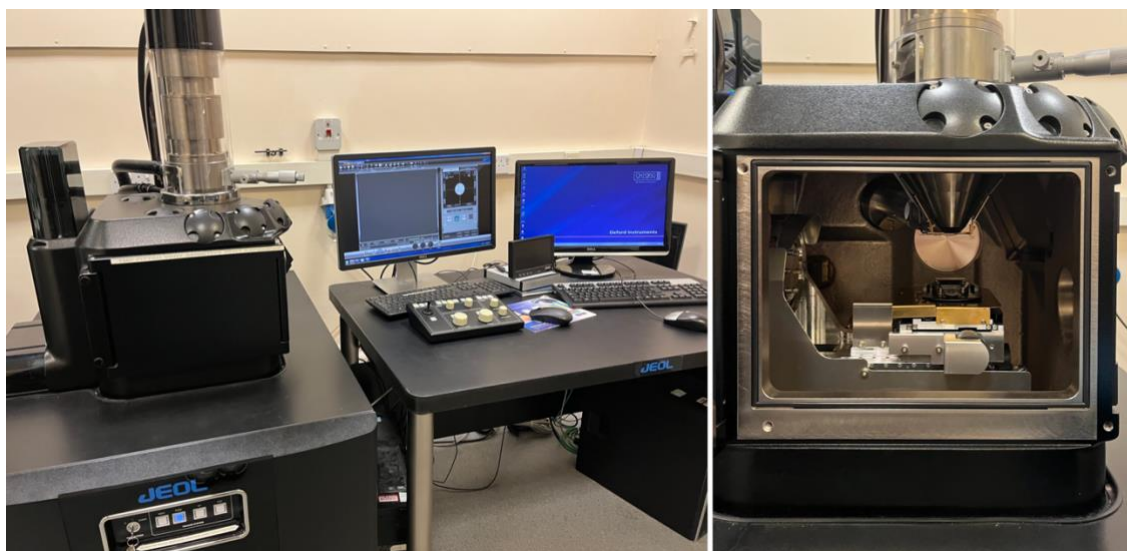
Figure 2.15: On the left, the full JEOL IT300 scanning electron microscope set-up and the computer to control the electron beam inside the chamber and capture images accordingly. On the right, inside the chamber, where the sample is inserted and held under vacuum.
