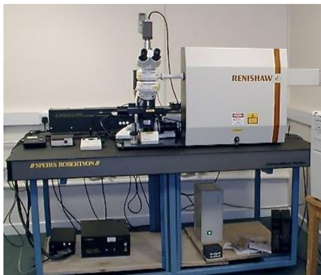
Figure 2.13: Renishaw 2000 laser Raman spectrometer with a green Ar + laser at a wavelength of 514nm. Implemented to determine presence of diamond and its purity. Image from 128 .
