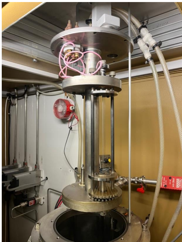
Figure 2.12: With the chamber lid lifted via the pneumatic, the wire carousel can be attached onto the filament, before the lid is lowered back into the chamber.
