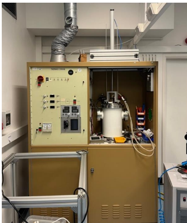
Figure 2.3: Full image of the Thomas Swan Reactor: the large chamber on the right and the operating panel on the left.
