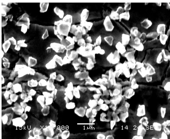
Figure 21 – <450nm acid washed, lithiated diamond assembled onto a tungsten substrate.
