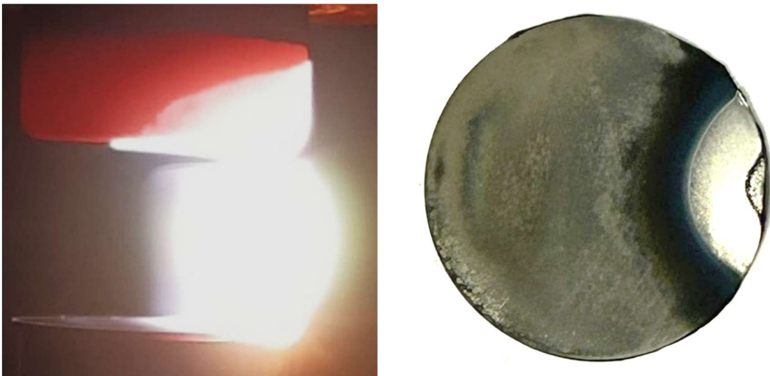
Figure 19 – On the left a plasma arc resulting from a 2° misalignment between electrodes Power: 1810 W Pressure: 180 Torr and resulting deposition on a 25 mm Mo substrate on the right.
