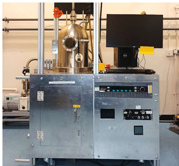
Figure 17 - The pulsed DC CVD reactor in the Bristol Diamond Laboratory, nicknamed 'The Minion'. The dome shaped growth chamber and computer used to run LabView and visible.
