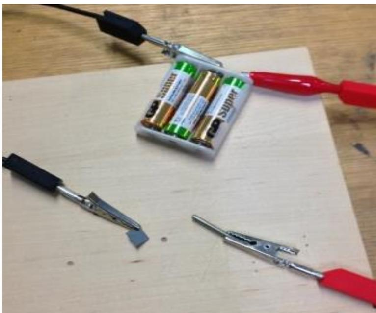
Figure 11. Electrochemical etching station for W.
