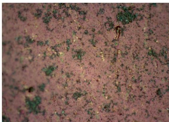
Optical Image W + Δ + O<sub>3</sub> + 0.5% HMW PEI + 0.5% BDD (A) after annealing (x100)
