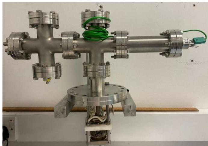
Figure 23 Image of the thermionic testing kit device.
