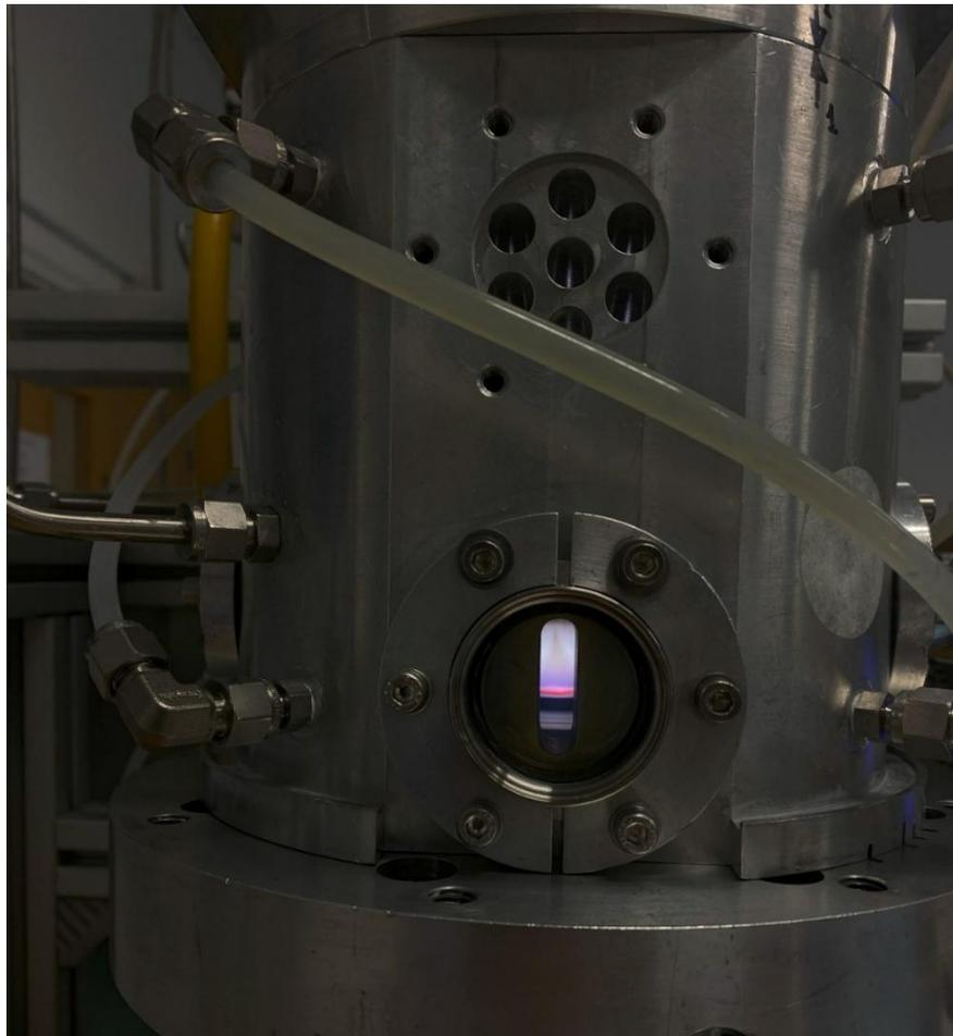
*Figure 6 The front MWCVD reactor growing nitrogen doped diamond (NND) on a molybdenum substrate at the University of Bristol Diamond Laboratory.*
