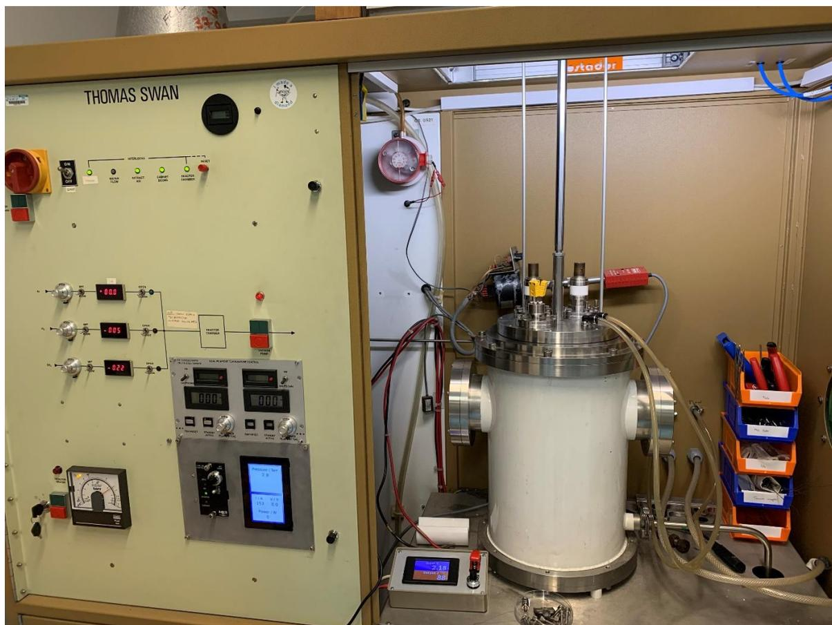
**Figure 24:** Modified large-area hot filament CVD reactor. (Left) The reactor control panel with pressure gauge, mass flow controllers and filament power controls. (Right) The stainless steel reactor casing.
