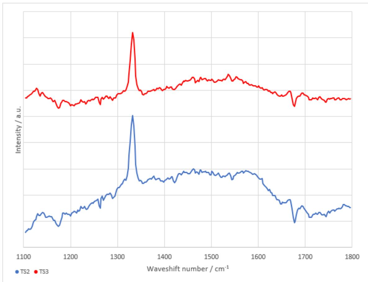
**Figure 28:** Raman spectrum from samples TS2 (blue) and TS3 (red) – diamond grown on a Si substrate. Single nano-diamond seeded sample, growth conditions 1 % CH<sub>4</sub> for 3 h, with 3 × 7.25 cm Ta filaments, 350 W. The diamond peaks for TS2 and TS3 were recorded at 1332 cm<sup>-1</sup>.
