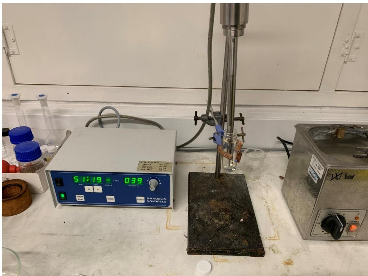
**Figure 23:** Ultra-sound probe used to prepare the diamond seeding solution.
