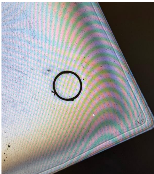
Figure 7 Diamond surface post laser etching.
