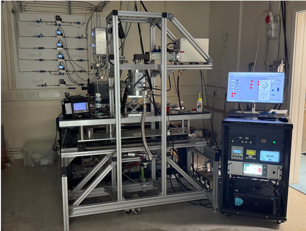
Figure 8 Microwave reactor used in Boron doping and hydrogen termination.
