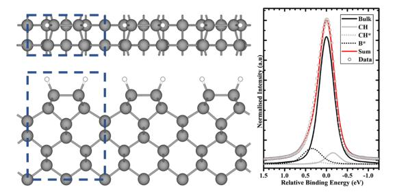
FIGURE 3.9: (a) The surface structure and top few layers of the (2x1) hydrogen terminated diamond surface, and (b) the corresponding C1s core level spectrum taken from Schenk *et al.*[33]
