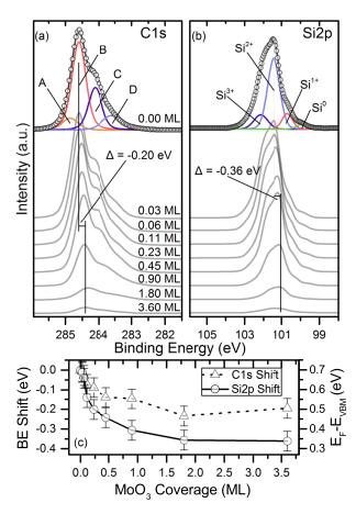
FIGURE 5.1: Details of the C1s ( $\hbar\omega = 350 \text{ eV}$ ) and Si2p ( $\hbar\omega = 150 \text{ eV}$ ) core levels acquired at each MoO<sub>3</sub> coverage. (a) and (b) show the fitting models applied to the C1s and Si2p core level respectively (only the respectively as a function of MoO<sub>3</sub> coverage and the position of the Fermi level relative to the diamond valence band maximum, based on the C1s position.[47]
