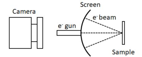
FIGURE 2.9: Simplified schematic of the elements of a low energy electron diffraction system.
