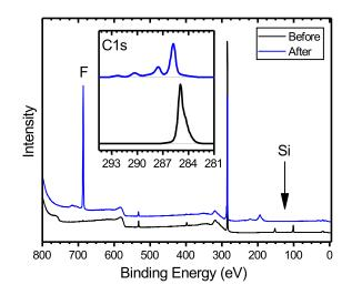
FIGURE 7.5:  $SF_6$  plasma treatment of silicon terminated diamond results in the removal of silicon and the formation of fluorinated diamond.
