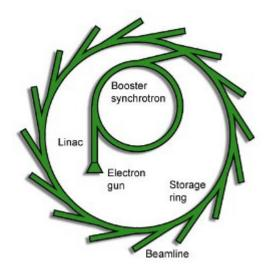
FIGURE 2.1: Schematic of the general structure of a modern synchrotron, showing the linear accelerator, booster ring, storage ring and beamlines. Taken from the Diamond website [9]
