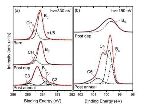
FIGURE 3.1: Carbon 1s and silicon 2p core level spectra of a (100) oriented diamond sample at various stages of silicon termination. Taken from Schenk *et al.* [4]
