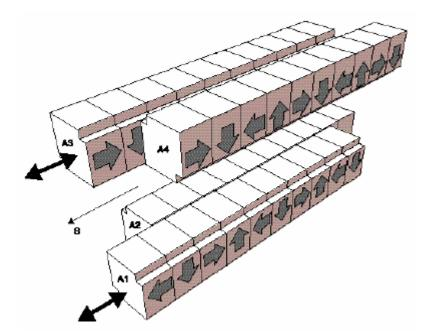
FIGURE 2.4: The four girder arrangement which comprises the AP-PLE II style undulator. From [13]
