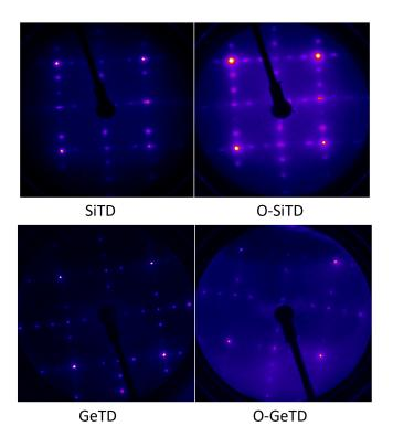
FIGURE 6.5: LEED patterns for pristine and oxidised Group IV terminated diamond surfaces. The rotation of the oxidised GeTD pattern relative to the pristine GeTD pattern is the result of remounting the sample after atmosphere exposure.
