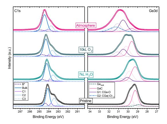
FIGURE 6.4: Germanium-terminated (100) diamond before (Pristine) and after exposure to  $H_2O$  or  $O_2$  *in situ*, and exposure to atmospheric conditions. Components are vertically offset from the spectra, and only the Ge3d<sub>5/2</sub> components are displayed, for clarity.
