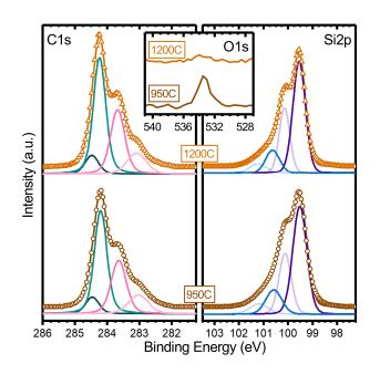
FIGURE 6.2: Fitted C1s and Si2p core level spectra obtained for a silicon-terminated diamond surface, (i) as-prepared and (ii) after a subsequent 1200°C anneal. Components are vertically offset from the spectra, and only the Si2p<sub>3/2</sub> components are displayed, for clarity. Inset shows the corresponding O1s core level from a survey scan
