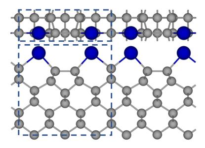
FIGURE 3.8: Our proposal for the structure of silicon terminated diamond (100). Top down view (top) and side view (bottom).
