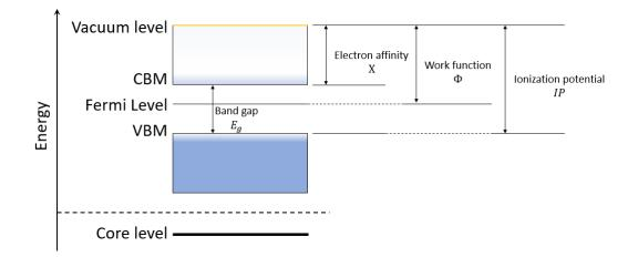
FIGURE 2.5: Schematic of the band structure of a semiconductor, showing graphical definitions of the important energies.
