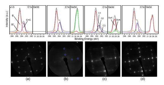
FIGURE 4.3: High resolution C1s (350 eV, left) and Ge3d (100 eV, right) photoemission spectra for Sample 2 at each processing step, with corresponding LEED patterns (70 eV), for (a) the bare (100) diamond surface; (b) after Ge deposition; (c) 500°C anneal, 75 minutes; (d) 950°C anneal, 20 minutes; components are again offset for clarity and a guide to the eye is given in (b)
