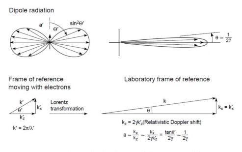
FIGURE 2.2: The angular distributions of photons emitted from an accelerated charge in the particle reference frame (left) and the laboratory frame (right). From [10]
