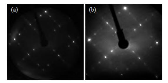
FIGURE 3.7: LEED patterns for silicon terminated diamond before (left) and after (right) oxidation by atmosphere exposure. Taken from Schenk *et al.* [19]
