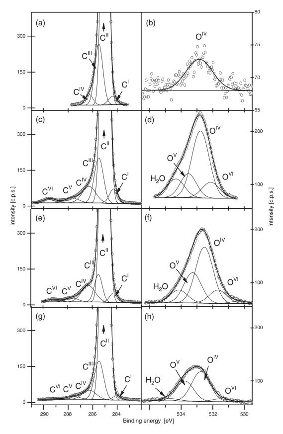
FIGURE 3.11: XPS spectra showing the mixture of states which result, regardless of oxidation method. The samples are UNCD, with C1s core level left, and O1s core level right. (a,b) H-terminated, (c,d) plasma oxidation, (e,f) piranha acid oxidation, (g,h) UV oxidation. Taken from Torrengo *et al.* [46]
