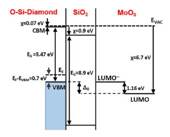
FIGURE 5.3: A schematic energy level diagram of the interface between the oxidised silicon terminated diamond and the MoO<sub>3</sub> LUMO.
