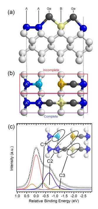
FIGURE 4.2: A schematic diagram of the top-down view, (a), and the side view, (b), of the possible structures of surface unit cells on C(100)- $(3 \times 1)$ :Ge, and a visual assignment of the C1s components is shown in (c). The outlined structures in (b) represent the co-existing, but not necessarily adjacent, complete and incomplete  $(3 \times 1)$  unit cells. A discussion of these structures is presented in the text.
