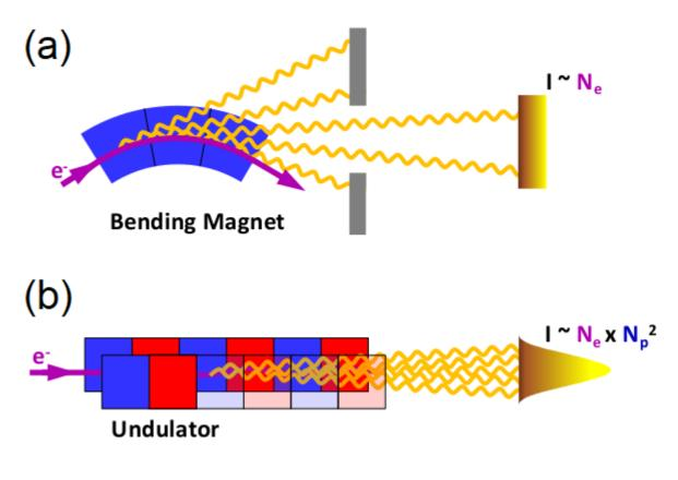
FIGURE 2.3: Bending magnet radiation (a) sweeps through a large angle, while undulator radiation (b) is confined to a smaller cone as a result of the electron path sweeping back and forth. Adapted from [12]
