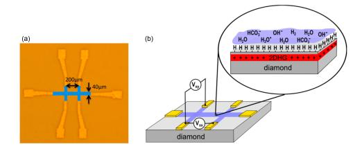
FIGURE 3.12: (a) Optical microscope image showing the Hall bar device fabricated on the diamond surface. The blue region indicates the area which is hydrogen terminated. (b) a schematic of the same device, with a zoomed image showing the induced conductivity in the presence of a water adlayer. Adapted from Figure 1 of Edmonds *et al.* [3]
