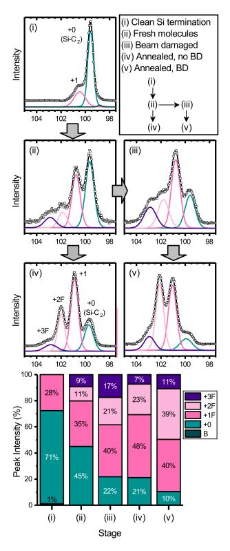
FIGURE 7.2: Evolution in core level appearance from silicon termination, through deposition of  $C_{60}F_{48}$ , exposure of  $C_{60}F_{48}$  to synchrotron radiation, and finally annealing.
