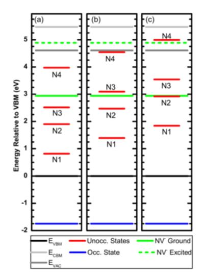
FIGURE 3.5: Silicon terminated diamond band structure models derived from ARPES and NEXAFS. (a) Assumes that the states seen in NEXAFS originate from the Bulk state in the C1s core level, (b) from the C1 state, (c) from the C2 state. Taken from Schenk *et al.* [18]
