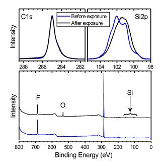
FIGURE 7.4: Atmosphere exposure of the incompletely fluorinated surface results in adsorption of oxygen and broadening of the silicon core level
