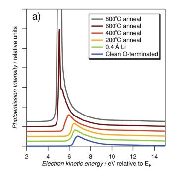
FIGURE 3.18: Shifts in photoelectron cutoff, followed by the formation of a large NEA peak, after a series of anneals of the lithiated oxygen terminated diamond surface. Taken from O'Donnell *et al.* [93]
