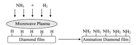
FIGURE 3.16: Conceptual schematic of microwave plasma amination. Taken from Wei *et al.*[59]
