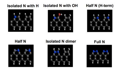
FIGURE 3.13: Some of the DFT calculated structures for a nitrogen terminated surface. Taken from Supplementary Figure 1 in Stacey *et* al.[52]
