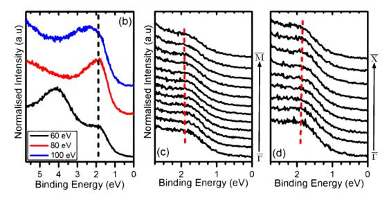
FIGURE 3.4: ARPES results showing the non-dispersive nature of the silicon terminated diamond surface state. Adapted from Figure 3 in Schenk *et al.*[18]
