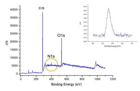
FIGURE 3.15: Survey spectrum demonstrating the relative nitrogen and oxygen coverages on an amine terminated diamond surface. Taken from Figure 3 of Suaebeh *et al.* [45]
