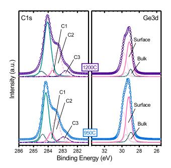
FIGURE 6.3: Fitted C1s and Ge3d core level spectra for a germaniumterminated diamond surface, as-prepared (bottom) and after a subsequent 1200°C anneal (top). Components are vertically offset from the spectra, and only the  $Ge3d_{5/2}$  components are displayed, for clarity.
