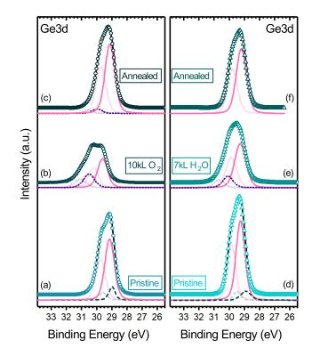
FIGURE 6.6: Ge3d spectra illustrating the thermal stability of the oxidized GeTD surface. (a,d) Pristine; exposed to (b) 10kL O<sub>2</sub>, (e) 7kL H<sub>2</sub>O; subsequently annealed for 15 minutes to (c) 700°C, (f) 300°C
