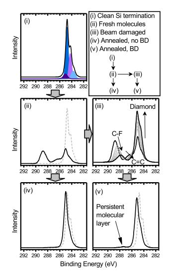
FIGURE 7.1: Evolution of the C1s core level throughout treatments, as detailed in text.
