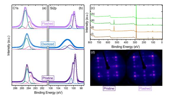
FIGURE 6.7: C1s (a) and Si2p (b) core level spectra demonstrating the thermal stability of the oxidized SiTD surface. Survey scans (c) show the clean (i), oxidized (ii), after being flashed twice at 1200°C (iii), and finally after two further flashes at 1400°C (iv); (d) LEED patterns corresponding to the pristine and post-treatments surface.
