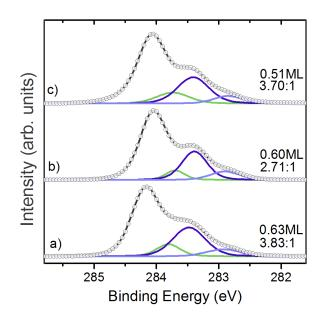
FIGURE 4.4: C1s spectra for 950°C annealed samples (bulk components omitted); (a) Sample 1, (b) Sample 2, (c) the low initial coverage sample; the corresponding germanium coverage and the C2:C3 ratio for each sample is included to the right of each spectrum.
