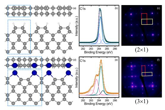
FIGURE 6.1: Schematic model with unit cell outlined, C1s x-ray photoelectron spectra ( $\hbar \omega = 350 \text{ eV}$ ) and LEED pattern for the (2 × 1) hydrogen terminated (a-c) and (3 × 1) silicon-terminated (d-f) diamond surfaces
