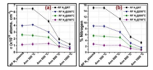
FIGURE 3.14: Plot demonstrating the low thermal stability of the nitrogen termination created. Taken from Figure 3 of Chandran *et al.*[53]
