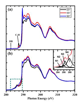
FIGURE 3.3: NEXAFS spectra for hydrogen (a) and silicon (b) terminated (100) diamond. Taken from Schenk *et al.* [18]
