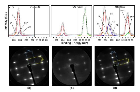
FIGURE 4.1: High resolution C1s (hv=350 eV, left panel) and Ge3d (hv=100 eV, right panel) photoemission spectra for Sample 1 at each processing step, with corresponding LEED patterns<sup>1</sup>(70 eV), for (a) C:H, (b) C:H + Ge deposited, (c) C:Ge - 950°C anneal; components have been offset for clarity.
