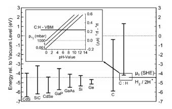
FIGURE 3.10: Diagram indicating the band gaps of a range of common semiconductors, relative to the vacuum level, and to the chemical potention for reduction of water. Taken from Maier *et al.*[2]
