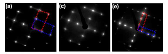
FIGURE 3.2: LEED patterns (70eV) throughout the silicon termination in Schenk *et al.* [4] Figure adapted from that paper. (a) Hydrogen terminated diamond, (c) after silicon deposition, (e) and after annealing.
