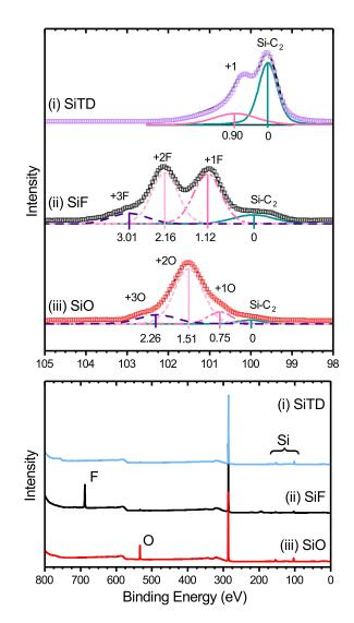
FIGURE 7.3: A comparison of the survey scans and fitting models employed for the Si2p core level of (i) pristine silicon-terminated diamond, (ii) fluorinated silicon-terminated diamond and (iii) oxidised silicon-terminated diamond.
