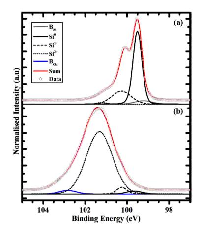
FIGURE 3.6: Silicon 2p core level spectrum for the clean and oxidized silicon termination explored in Schenk *et al.* [19] Adapted from Figure 6.
