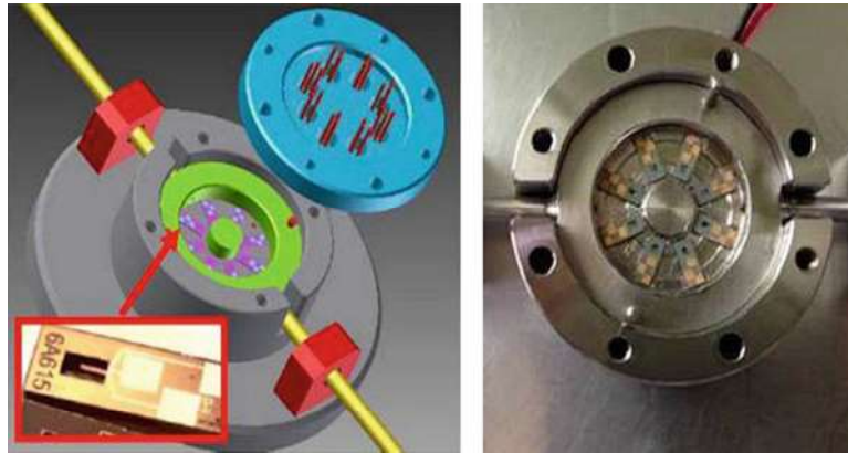
Fig. 12.5 Left: Three-dimensional drawing of an EN gas sensor showing the 8 MEMS cantilevers inside. Right: Photograph of the sensor. (Figure reproduced from Ref. [71] under CC BY 4.0 licence)
