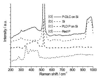
**FIGURE 3** Details of the 200–1000 cm<sup>-1</sup> regions of Raman spectra (514.5-nm excitation) of (**a**) a P-DLC film deposited on Si at  $T_{sub} = 25$  °C following PLA of a 50% P in C target in vacuum, (**b**) a bare Si substrate, (**c**) a thin film of phosphorus deposited on Si by PLD and (**d**) a sample of pure red phosphorus. The four spectra have been offset vertically for clarity
