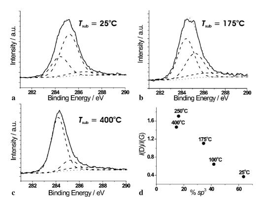
**FIGURE 4** Detailed views of the C(1s) peak in the XPS spectra of P-DLC films deposited at  $T_{sub} = 25 \,^{\circ}$ C (a), 175  $^{\circ}$ C (b) and 400  $^{\circ}$ C (c), together with the respective deconvolutions into three Voigt line shape functions. **d** Plot of I(D)/I(G) ratio (from Fig. 2d) and C-sp<sup>3</sup> content for films grown at a range of different  $T_{sub}$ values
