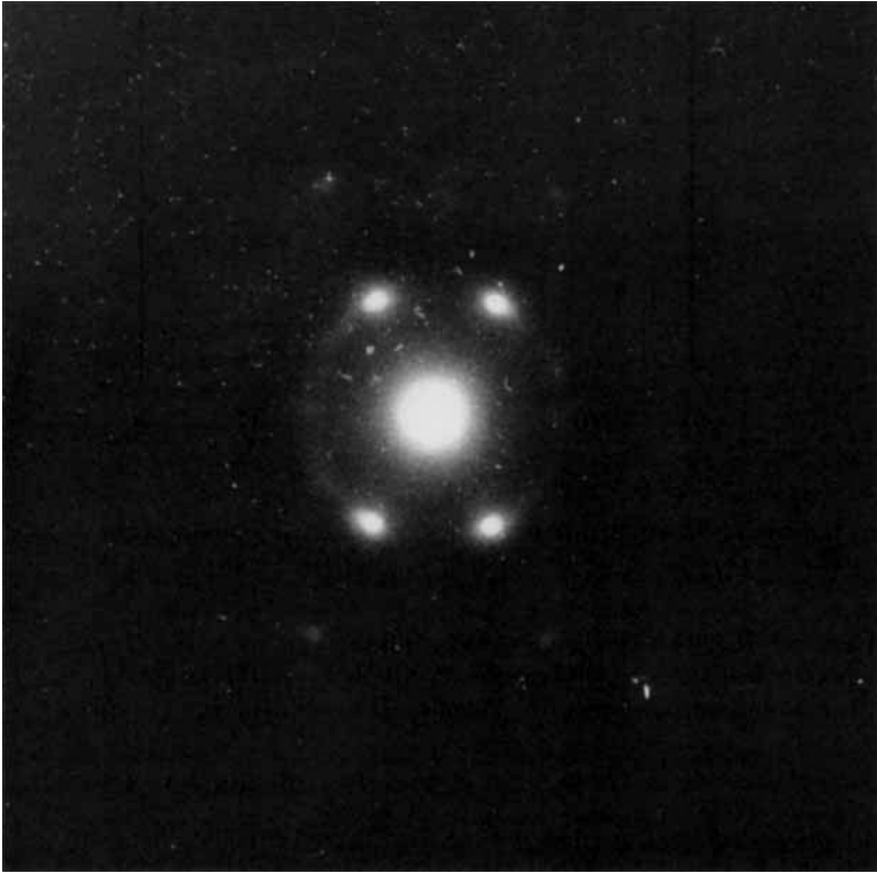
Fig. 3. Electron diffraction pattern of a single nanocrystalline diamond cluster embedded in the amorphous diamond film matrix (100 nm thickness) lifted from a silicon substrate by HF
