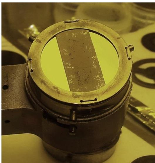
Figure 6.1: Custom-made sample holder used to hold Li-N co-doped diamond film grown on W substrate for thermionic emission experiment.
