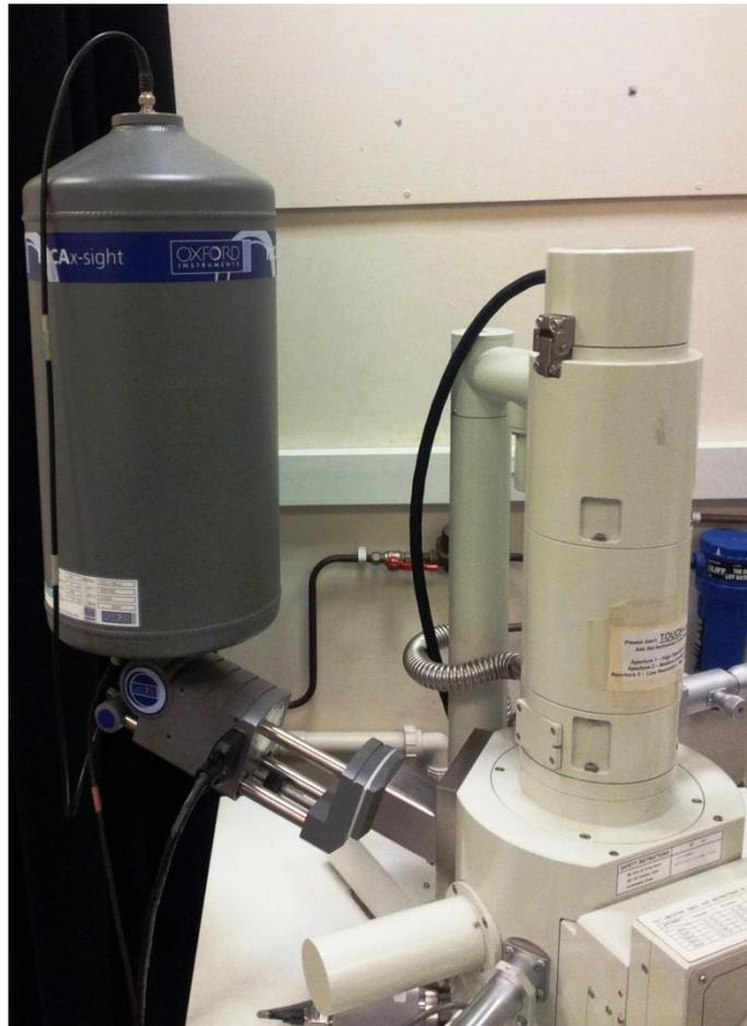
Figure 2.6: EDX analyser attached to JEOL JSM 5600LV in the Electron Microscope Unit, School of Chemistry, University of Bristol.
