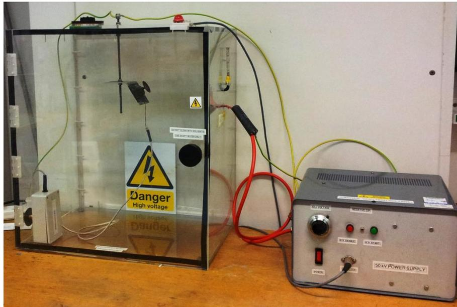
Figure 1.6: The electro spray instrument used in Diamond Laboratory, University of Bristol for diamond seeding process.
