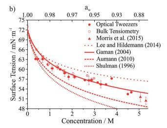
Fig. 4 Surface tension measurements on two atmospherically relevant systems: (a) sodium chloride and (b) glutaric acid. Also included are bulk tensiometry measurements, E-AIM modeling (sodium chloride), surface tension parametrizations performed by others (glutaric acid), $^{47-50}$  and measurements on submicron aerosol using atomic force microscopy. $^{28}$  The upper axis gives water activity ( $a_{\rm w}$ ), which is inferred from the solute concentration.
