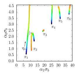
FIG. 4. Pole structure of a two component hard sphere fluid treated in the PY approximation for size ratio q=0.648 and fixed  $\eta_s+\eta_b=0.5$ . The colour indicates the value of the packing fraction  $\eta_s$  increasing from blue  $\eta_s=0.01$  to red  $\eta_s=0.49$ . Crossover occurs at  $\eta_s=0.28$  where  $\alpha_0\sigma_b=2.3$ , as indicated by the horizontal arrow.
