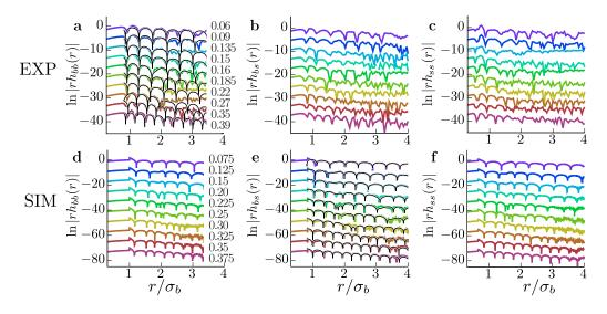
FIG. 3. Plots of  $\ln |rh_{ij}(r)|$  obtained by experiment (top) and simulation (bottom) for big-big, big-small, and small-small total correlation functions. The packing fraction  $\eta_s$  (marked) is increasing from top (blue) to bottom (red) for each case. Curves are shifted vertically for clarity. The black lines in (a) and (e) are fits from which  $\alpha_0$ ,  $\alpha'_0$ ,  $\alpha_1$ , and  $\alpha'_1$  in Eq. (5) are obtained. The simulations correspond to size ratio q = 0.648.
